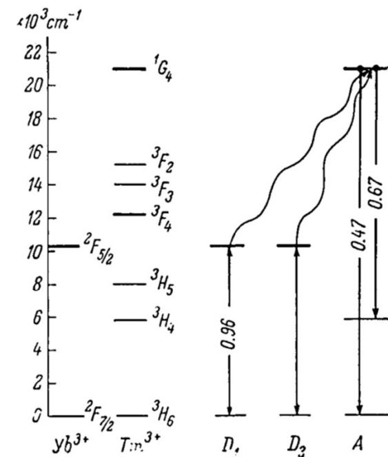
Fig. 4. Term diagram of Yb<sup>3+</sup> and Tm<sup>3+</sup> ions and cooperative sensitization by Yb<sup>3+</sup> ions of Tm<sup>3+</sup> emission.
