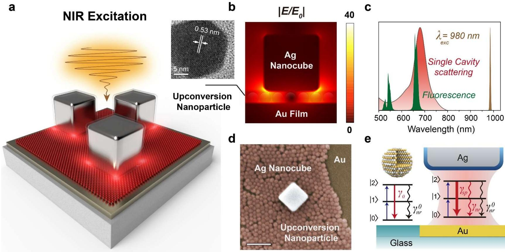
UCNP/plasmonic cavity hybrid comprising a gold film-coupled Ag nanocube with a sandwiched monolayer of UCNPs.
